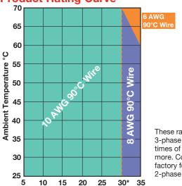
These ratings apply to 3-phase units with cycle times of 30 seconds or more. Consult the factory for 1- and 2-phase unit ratings.
