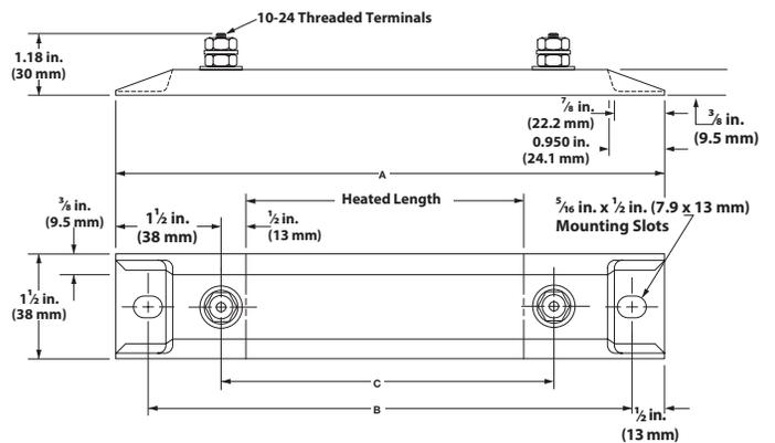
Two 10-24 threaded post terminals are placed one on each end.
