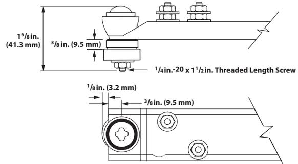
Insulators are suitable when air heating and/or voltage to ground is a concern. A secondary insulation bushing kit, part number **Z5230**, contains one set of bushings for one heater. To accommodate bushings,  $\frac{17}{32} \times \frac{11}{16}$  inch diameter mounting holes **must** be specified when ordering the heater.
