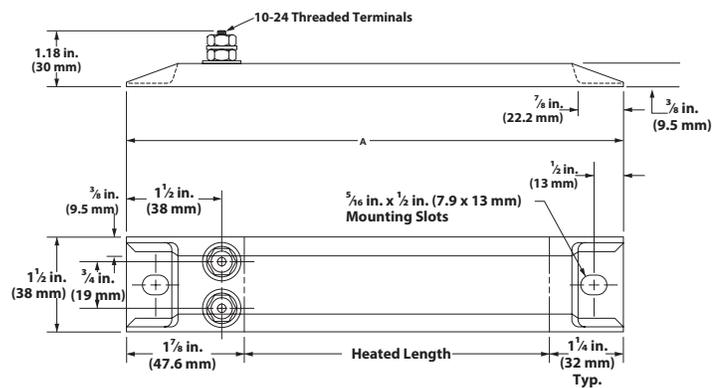
Two 10-24 threaded post terminals are used; both terminals on one end.
