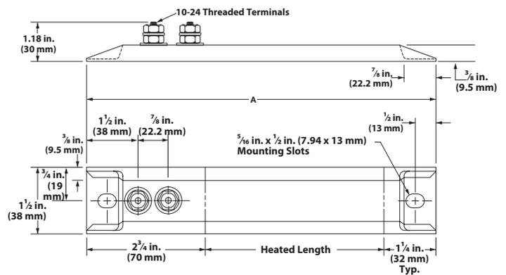
Two 10-24 threaded post terminals are in-line with each other on the same end.
