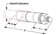
Ceramic-to-metal end-seals with threaded stud terminations provide an air-tight seal for continuous terminal temperatures up to 500°F (260°C). Watlow does not recommend this seal if terminations are exposed to temperatures exceeding 500°F (260°C).
