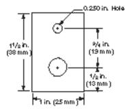
A 1½ in. (38 mm) x 1 in. (25 mm) wide x 16 gauge stainless steel bracket with one element hole and one mounting hole  $\frac{1}{2}$  in. (13 mm) from end.
