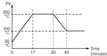
**Note:** When the ramp function is used, the lower display will show the current ramping value. However it will revert to show the set point value as soon as the up or down key is touched for adjustment. The ramp rate is initiated at power on and/or when the Set point is changed. Setting the RR setting to zero means no ramping function at all.
