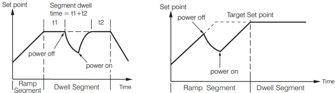
**Power failure recovery from PV at Dwell segment** **Power failure recovery from PV at Ramp Segment**
