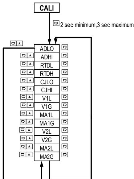
Press key for 2 seconds or longer (not more than 3 seconds) then release it to enter calibration Mode.
