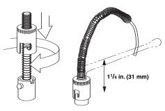
A thermowell allows you to use a thermocouple with a bayonet fitting to monitor heater temperature. The thermowell is located on the back of the panel to allow easy access for thermocouple replacement. Spring tension holds the tip of the thermocouple in contact for close control of the heater temperature. Thermocouple not included.
