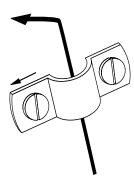
A thermocouple mounting clamp can be provided on the end of the heater case. The clamp is suitable for use with ½ inch (3.175 mm) and ½ inch (6.35 mm) O.D. sheath thermocouples, which should be bent 90° so that the sensing tip is just above and lightly touching the hot face at an element location.
