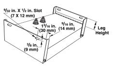
Standard ¼-20 X 1 ½ inch (M6-1 X 40) steel studs are welded to the case. For best support, studs should be approximately located on 12 inch centers. Consult Watlow for exact locations on specific heaters.
