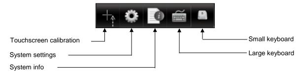
The Touchscreen Calibration icon is present only on units without DIP switches.
