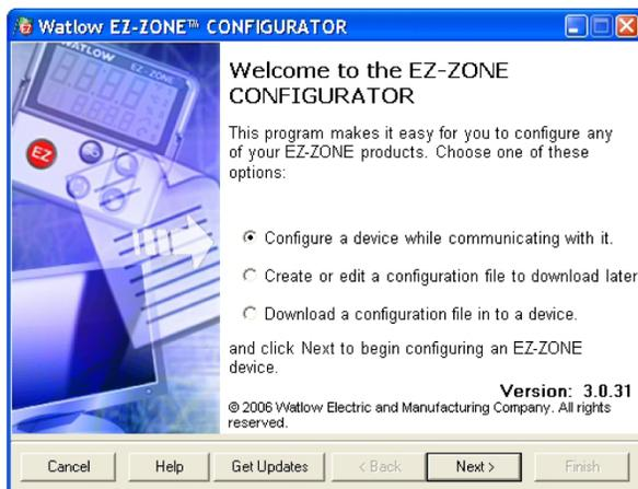
The EZ-ZONE configurator software is used to set up Watlow EZ-ZONE products in one simple process. It works without requiring the purchase of any communication options because it uses the standard bus communications protocol that is included with all EZ-ZONE products. EZ-ZONE configurator can be used for on-line and off-line configurations and downloading previously saved setups. It is available as a FREE download at [www.watlow.com](http://www.watlow.com).
