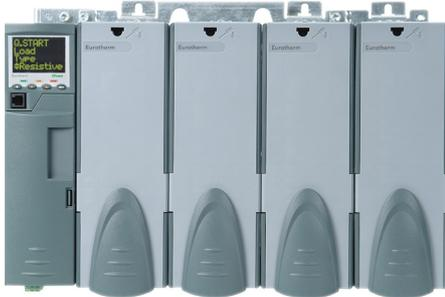
The EPower™ Advanced SCR Power Controller is a modular multi-channel SCR power controller unit. The EPower current ratings cover ranges from 50 Amps up to 630 Amps (compact variants) and from 800 Amps to 4000 Amps (MC EPower with HPower variants). The voltage rating can go up to a maximum of 690 volts depending on current variants.
