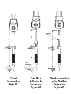
Plastic melt bolt thermocouples are designed so that the sensitive closed end portion of the tip can be inserted directly into the plastic stream of an extruder or injection molding machine. The measuring junction is thermally isolated from the metal bolt mass, assuring accurate reading of the melt temperature up to 260°C (500°F) continuous. Bolt is 300 series stainless steel.
