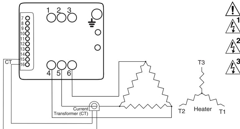
**3-phase, 3-leg Current Transformer Wiring**
