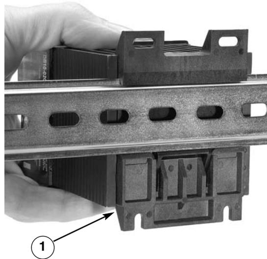
1. Press down on the release tab while rotating the unit up and away from the rail.
