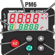
Upon power-up, the upper display will briefly indicate the firmware revision and the lower display will show PMb. The "b" in this case, reflects the B in the model number.
