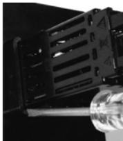
Place the blade of a screwdriver in the notch of the mounting collar assembly.
