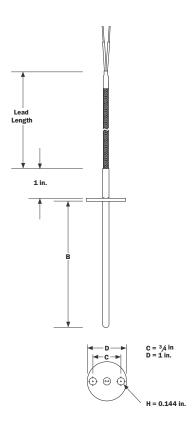
The flanged thermocouple allows rapid assembly and low profile when going through bulkheads.
