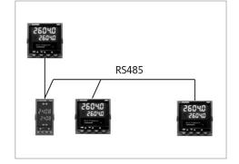
Master Modbus communications significantly increases the applications open to the 2604 controller. In its simplest form it can be used to retransmit a setpoint to a number of slave controllers in a multi-zone furnace.
