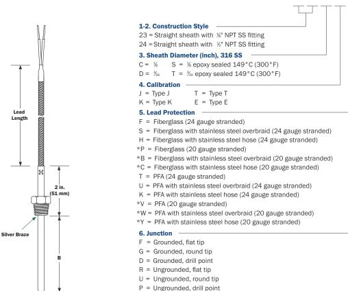
Rigid sheath with threaded fitting provides accurate placement in process applications.
