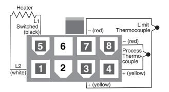
Thermocouple and heater connector
