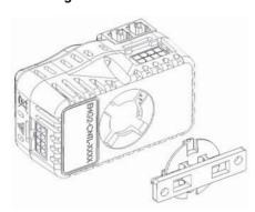
The Series EHG CL mounting bracket lets you mount the controller in any of four angles. After disconnecting both wiring connectors, gently rotate the controller counterclockwise until it unlocks from the mounting bracket. Re-orient the controller on the mounting bracket and gently rotate it clockwise until it locks.
