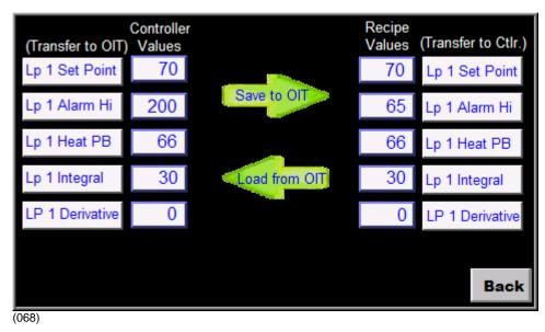
Optional: The values in the RW addresses are automatically saved in non-volatile memory every five minutes, but adding a button that momentarily sets LB-9029 forces the values to be saved and can avoid lost data in the event the power is shut off too soon after editing a recipe.
