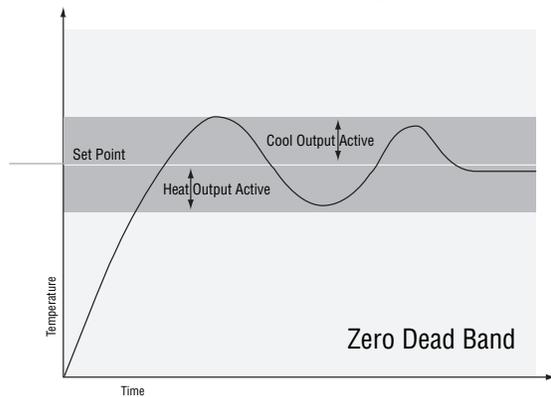
When the **dead band value is a negative value**, both heating and cooling outputs are active when the temperature is near the set point.
