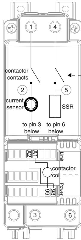
Internal wiring in an ST with a double-pole contactor without a limit (ST \_ B - F \_ \_ \_ \_ \_).
