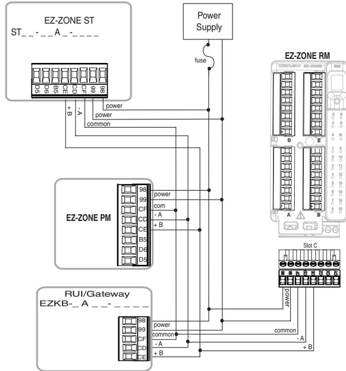
**A network with all devices configured using Modbus RTU.**
