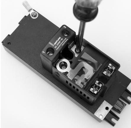
2. With a Phillips screwdriver, remove the four nearest screws that were under the module.
