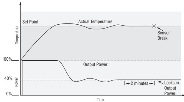
Input Error Latching (**IER**) (Setup Page, Analog Input Menu) determines the controller’s response once a valid input signal returns to the controller. If latching is on, then the controller will continue to indicate an input error until the error is cleared. To clear a latched alarm, press the Advance Key **⏏** then the Up Key **⬆**.
