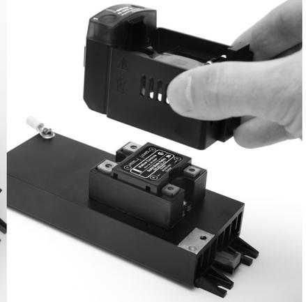
3. Lift the controller body, exposing the solid-state relay.
