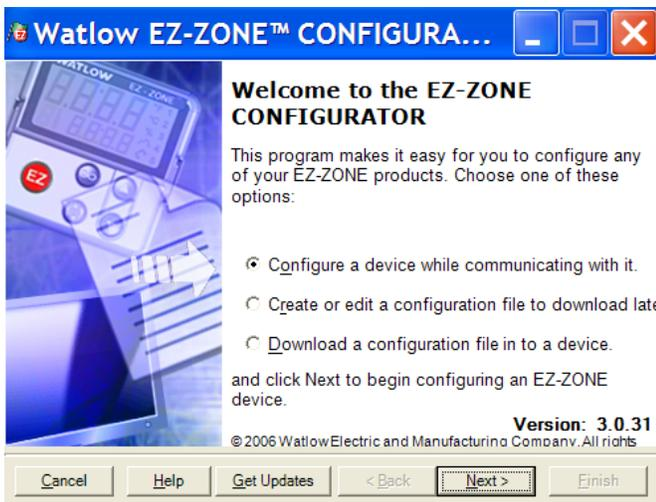
If the PC is already physically connected to the EZ-ZONE ST control click the next button to go on-line.
