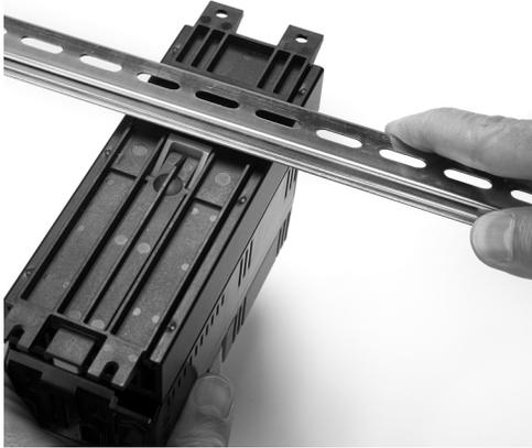
To mount the controller on a DIN rail, first hook the top flange on the back of the heat sink on to the top of the DIN rail. Then rotate the controller to an upright position until the lower flange snaps into place.
