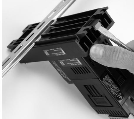
To dismount the controller, first use a screwdriver to pull down the small lever on the bottom of the heat sink and rotate the bottom of the controller forward. Then lift the the controller off of the rail.
