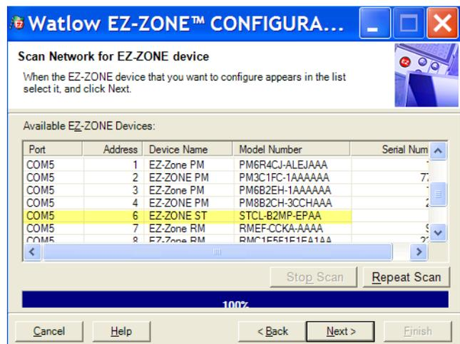
In the previous screen shot the ST is shown highlighted to bring greater clarity to the control in focus. Any EZ-ZONE device on the network will appear in this window and would be available for the purpose of configuration. After clicking on the control of choice simply click the next button once again. The next screen appears below.
