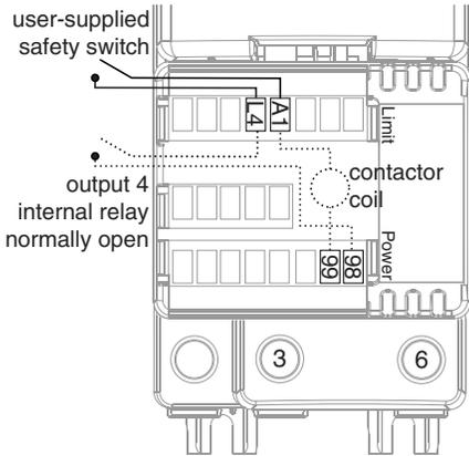
You may remove the factory-installed jumper between A1 and L4 to install a safety switch for the limit relay (ST \_ L - \_ \_ \_ \_ \_).
