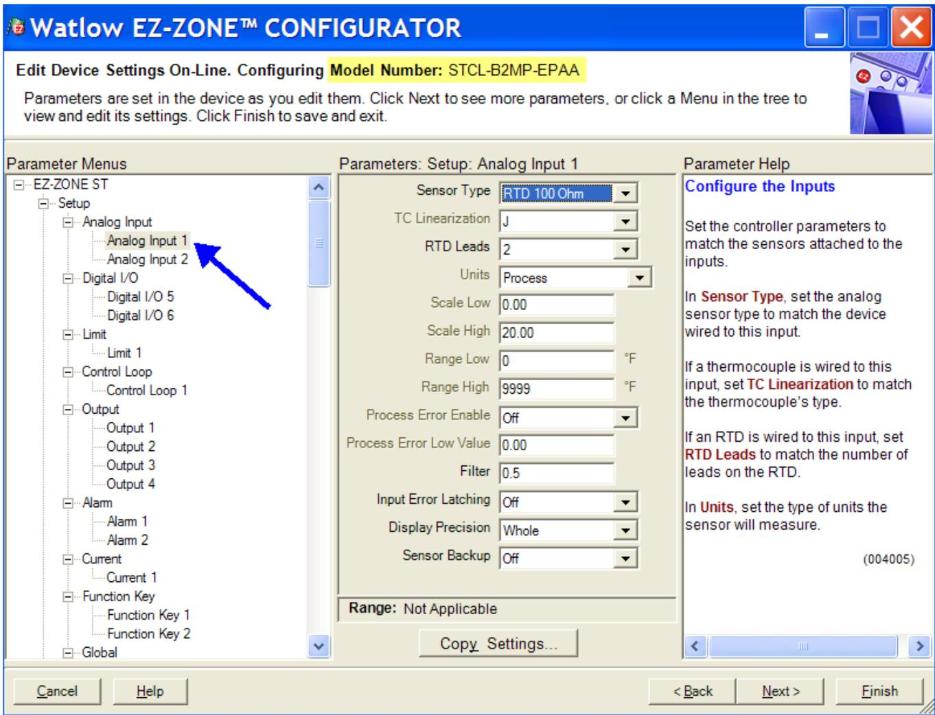
In the screen shot above notice that the device part number is clearly displayed at the top of the page (yellow highlight added for emphasis). When multiple EZ-ZONE devices are on the network it is important that the part number be noted prior to configuring so as to avoid making unwanted configuration changes to another control.
