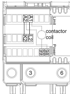
You can use output 2 (L2 and K2) to deactivate the contactor coil on an ST without a limit (ST \_ B - \_ \_ \_ \_ \_).
