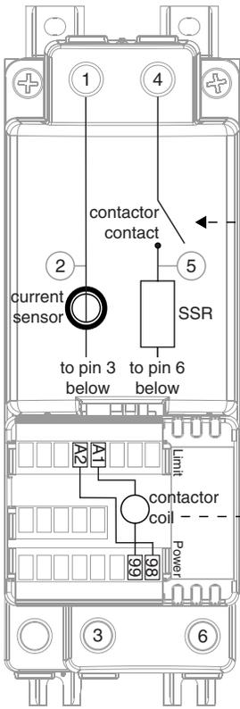
Internal wiring in an ST with a single-pole contactor without a limit (ST \_ B - B \_ \_ \_ \_ \_).
