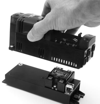
4. Lift the controller body, exposing the solid-state relay.
