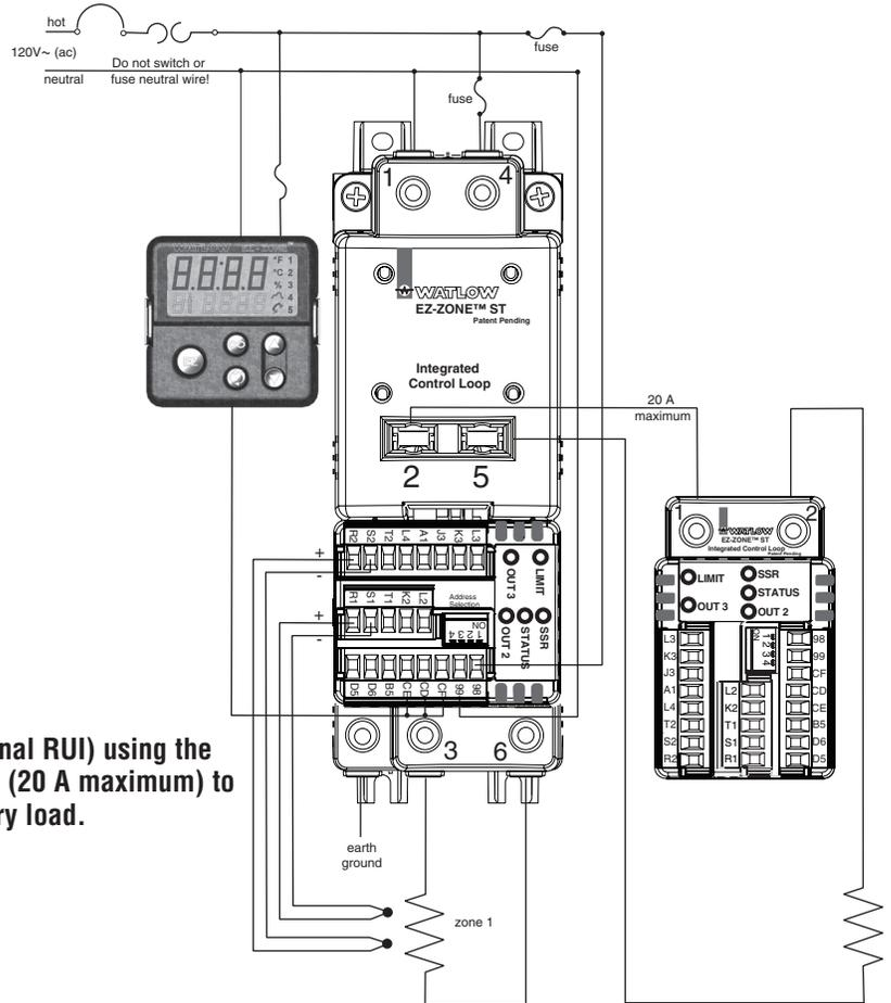
System (with optional RUI) using the auxiliary terminals (20 A maximum) to operate a secondary load.
