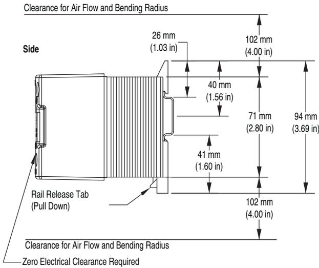
**!** Mount the cooling fins vertically. Failure to do so may cause premature unit failure.
