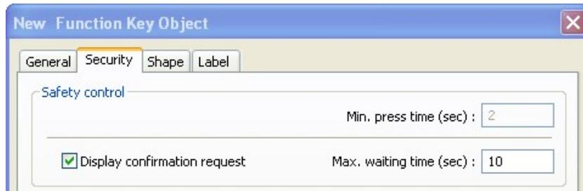
**Min. press time (sec):** This sets the minimum amount of time in seconds that the object needs to be pressed in order to activate it.
