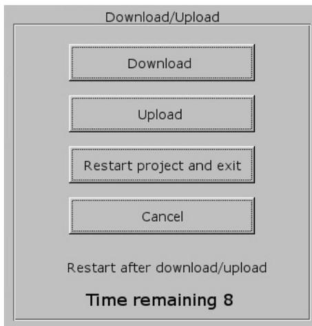
2. Select **Upload**. In the Upload Settings window, select **Upload all project files** and enter the Upload password (111111 is the default).
