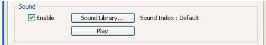
The default sound is the HMI's beep. For models equipped with an audio output jack, you can select other sounds from the sound libraries to play when the object is activated.
