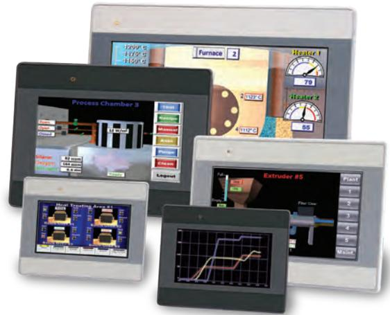
The Silver Series EM is a rugged, touch-screen operator interface terminal (OIT). Available in three sizes (4.3, 7 and 10 inch diagonal display sizes), the OITs feature serial and Ethernet communications with multiple controllers, email messaging, universal serial bus (USB host), data logging, flexible password security and multiple languages. The small bezel size and two-inch depth make mounting in tight spots easy.
