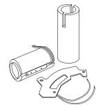
To increase heating efficiency of your application, silicone rubber heaters can be thermally insulated with silicone sponge rubber bonded to one side in the following thicknesses: 1/16, 1/8, 1/4, 3/8 or 1/2 in. (1.6, 3.2, 6, 9.5 or 13 mm).
