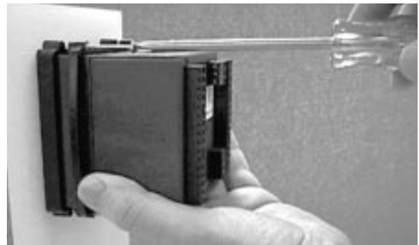
Figure 11.3b — Tightening the Screws.
