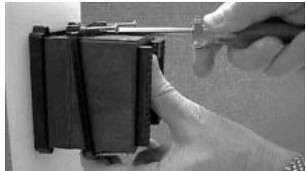
Figure 11.3c — Disengaging the Mounting Bracket.
