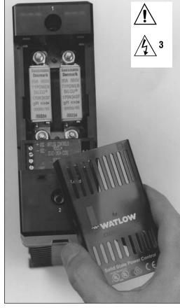
After removing all power, use a 7/16-inch nut driver to remove fuse mounting nuts. Torque to 4.52 Nm (40 in-lb).
