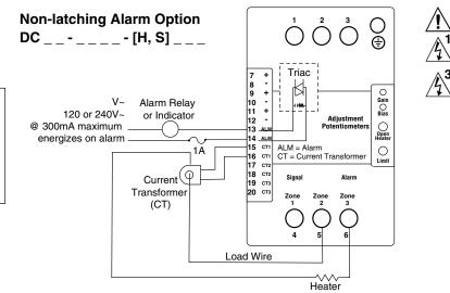
The Watlow DIN-A-MITE alarm option provides a common alarm output for open-heater or shorted SCR conditions. **This is a non-latching alarm.**
