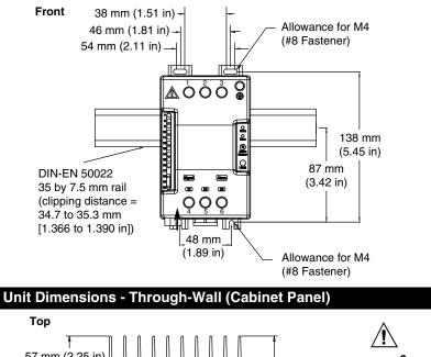
102 mm (4.0 in) clearance for air flow and wire bending radius
