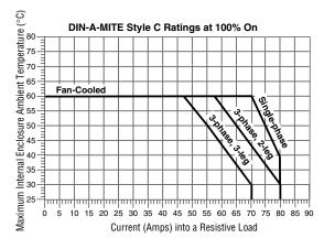
DIN-A-MITE Style C Ratings at 100% On
