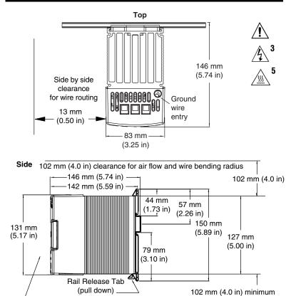
Front panel is touch-safe, no clearance is required.
