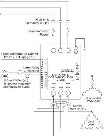
Non-latching Alarm Option (models DC\_\_-\_S\_-H\_\_\_\_)
