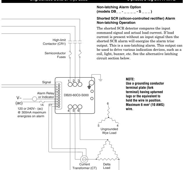
NOTE: The current transformer must be in the center uncontrolled leg on a 2-leg DIN-A-MITE.
