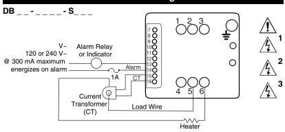
The Watlow DIN-A-MITE alarm option provides a common alarm output for shorted SCR conditions. **This is a non-latching alarm.**
