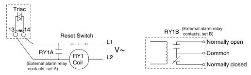
**Latching Alarm Relay Circuit**
