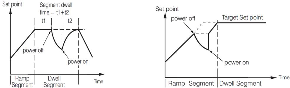
**Power failure recovery from profile at Dwell segment** **Power failure recovery from profile at Ramp segment**
