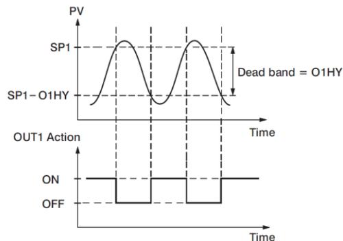
ON-OFF control may cause excessive process oscillations even if the hysteresis is set to the smallest value. If ON-OFF control is set (i.e. PB = 0), TI, TD, CYC1, OFST, CYC2, CPB, DB will no longer be applicable and will be hidden. Auto-Tuning mode and Bumpless transfer will also be unavailable.
