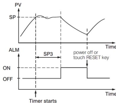
After the timer has finished, the dwell timer can be restarted by pressing the RESET key. The timer stops counting during manual control mode, failure mode, calibration and Auto-
