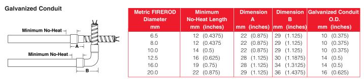
Galvanized conduit equals stainless steel hose in its abrasion protection. The conduit is attached with 90 degree elbow copper coupler that overlaps the heater sheath.
