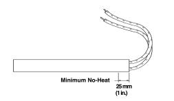
Swaged-in flexible leads, with a silicone-fiberglass insulation, are recommended for applications in which the leads must be bent at the exit point from the heater. Unless longer length is specified, 250 mm (10 inch) leads are supplied.
