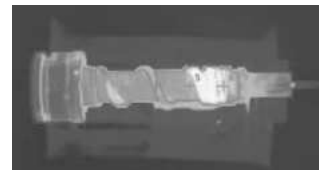
Temperature distribution using standard coiled cable heater.
